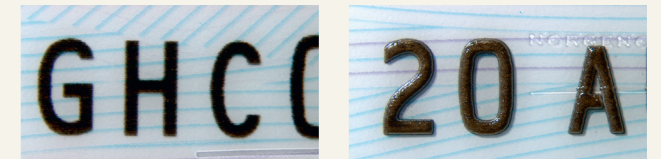
Personalization All personalization is laser engraved. The expiry date on the card's front, and the identity no. on the rear side have a tactile relief effect.
